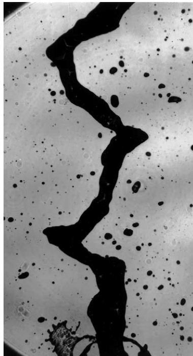
Fig. 4. Pulsed shadowgraph of large cross stream distortions near the tip of a turbulent round liquid jet at a large Weber number: water jet in still air, d = 4.8 mm, Re = 97,100 , We = 33,100 at a distance of 1040 mm from the jet exit.
