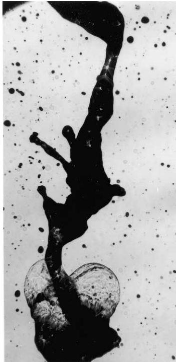
Fig. 5. Pulsed shadowgraph of bag-like breakup of large cross stream distortions near the tip of a turbulent round liquid jet at a large Weber number: water jet in still air, d = 4.8 mm, Re = 97,100 and We = 33,100 at a distance of 1040 mm from the jet exit.
